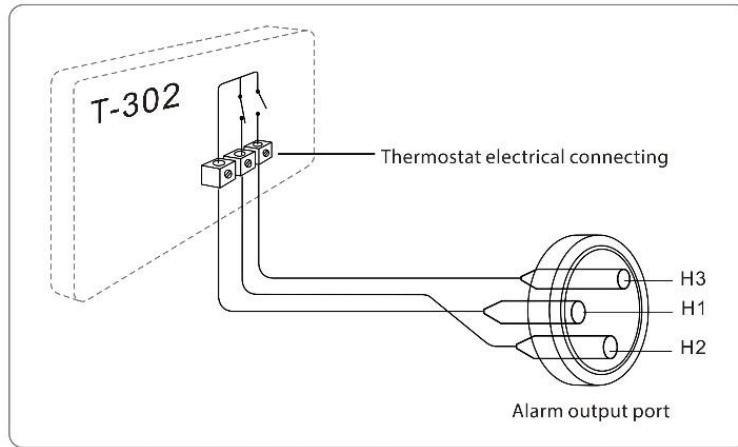
Note: The alarm output port is connected with a set of normally open and normally closed contacts of the relay inside the machine. The working current should be smaller than 3A while the working voltage should be smaller than 300V.
